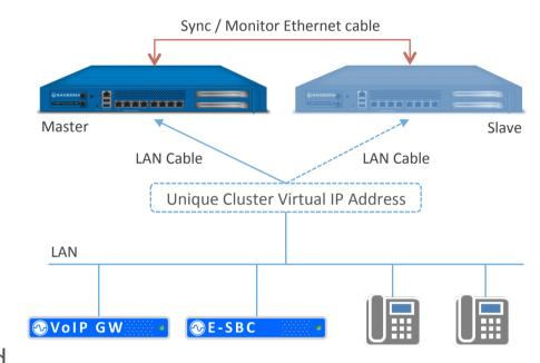
SIP phones, Gateways, SBCs are automatically directed to an active PBXACT server. No technician intervention required
